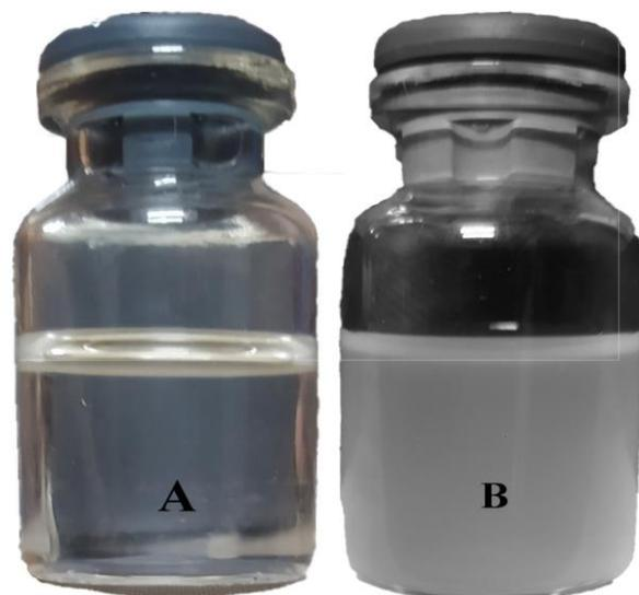
**Figure 1:** (A) collagen solution; (B) collagen-NPs solution (white turbidity)
