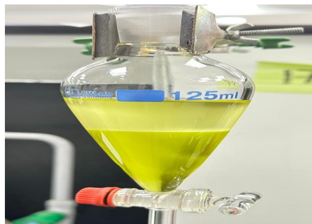
Figure 5: Biodiesel and glycerol formed after transesterification from selected promising green algal species Nannochloropsis oculata .
